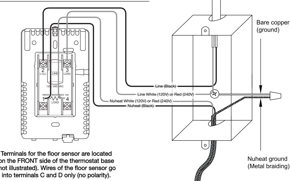
on the FRONT side of the thermostat base (not illustrated). Wires of the floor sensor go into terminals C and D only (no polarity).
