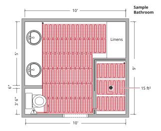
Select the Mesh kit that is no larger than the heated area. The heated area is the area of the floor that does not include permanent fixtures such as cabinets, toilets, sinks or tubs. The selected kit can be configured on the jobsite to fit the shape of the area to be heated.
