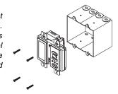
Mount the thermostat onto the electrical box using the provided screws.
