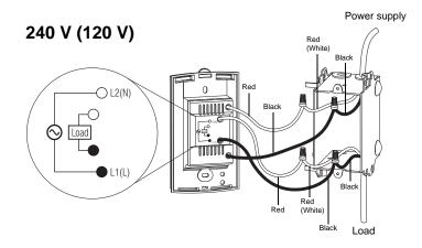
**NOTE**: All wires and connections must conform to the local electrical code. This thermostat has tinned copper wires for line and load connections. Special CO/ALR solderless connectors must be used if these wires are to be connected to aluminium conductors.
