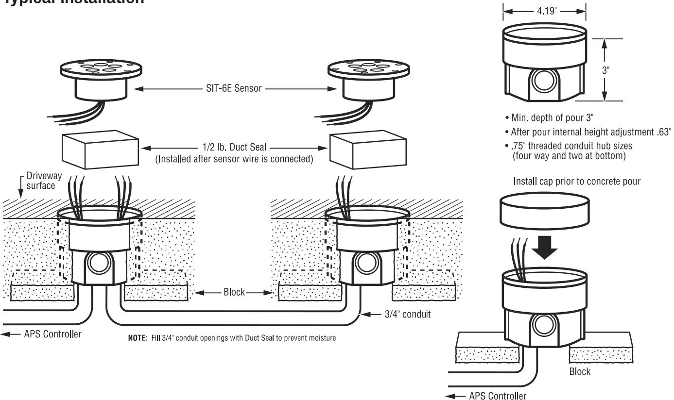
**NOTE:** The output signal of an SIT-6E pavement sensor is not a contact closure — it is a solid state switch compatible only with ETI's APS series and EUR-5A Control Panels. If a contact closure is desired for an output signal, please select from our HSC series of pavement sensors.
