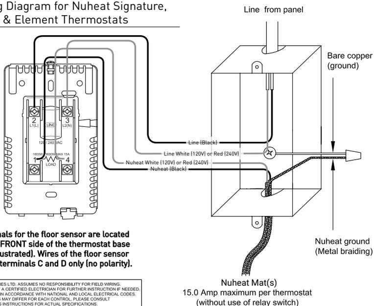
**Terminals for the floor sensor are located on the FRONT side of the thermostat base (not illustrated). Wires of the floor sensor go into terminals C and D only (no polarity).**
