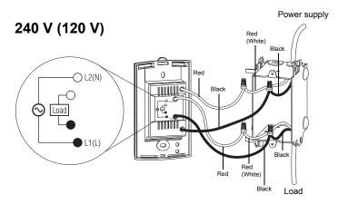
**NOTE**: All wires and connections must conform to the local electrical code. This thermostat has tinned copper wires for line and load connections. Special CO/ALR solderless connectors must be used if these wires are to be connected to aluminium conductors.
