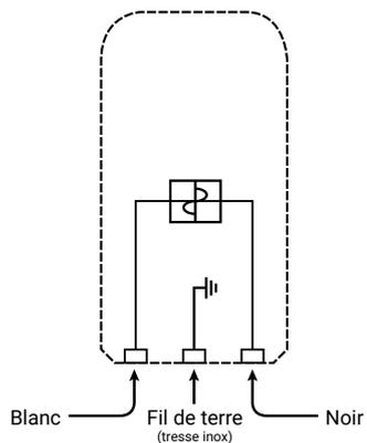
nVent NUHEAT Install Pro Alarm instructions de câblage (240V)
